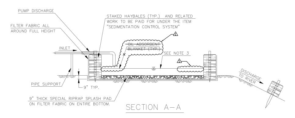
TEMPORARY SEDIMENT BASIN FOR DEWATERING DISCHARGE
